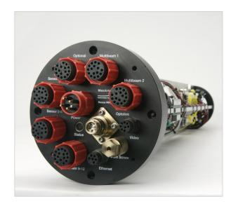
The MacArtney NEXUS MK V multiplexer is based on the Focal 907 video/data multiplexer combined with the MiniController, Ethernet converters and the Focal Gb-media converters. Power switching of all sensors and cameras is software controlled and combined with monitoring of sensor power status.
